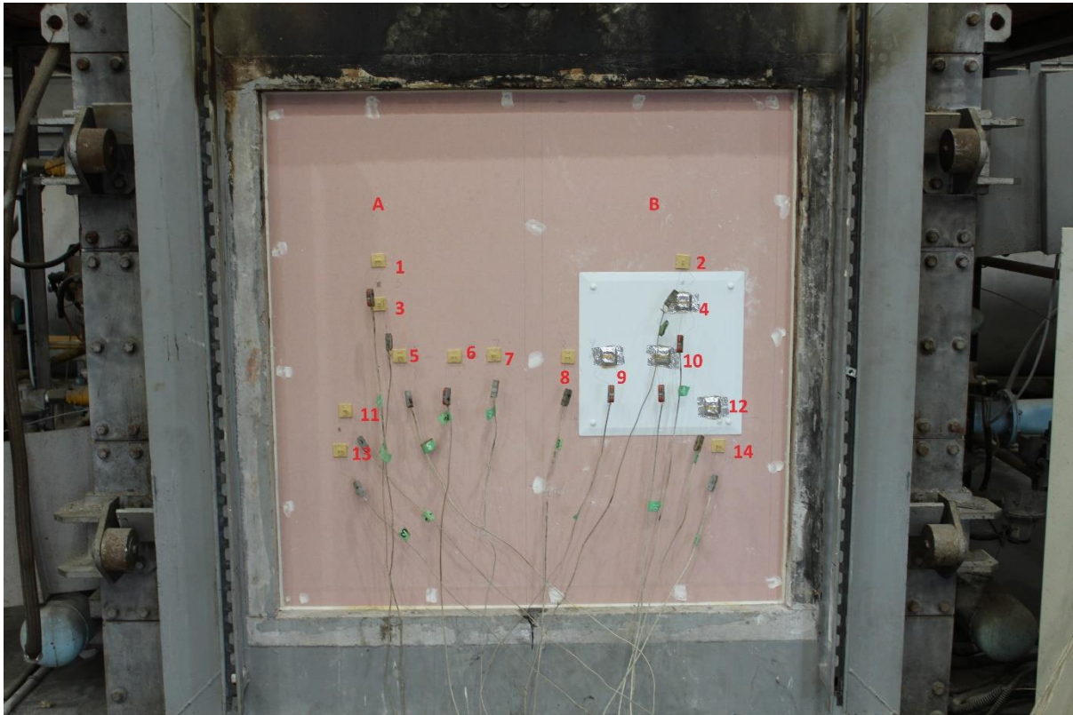
Figure 3 – Unexposed face Thermocouples location
