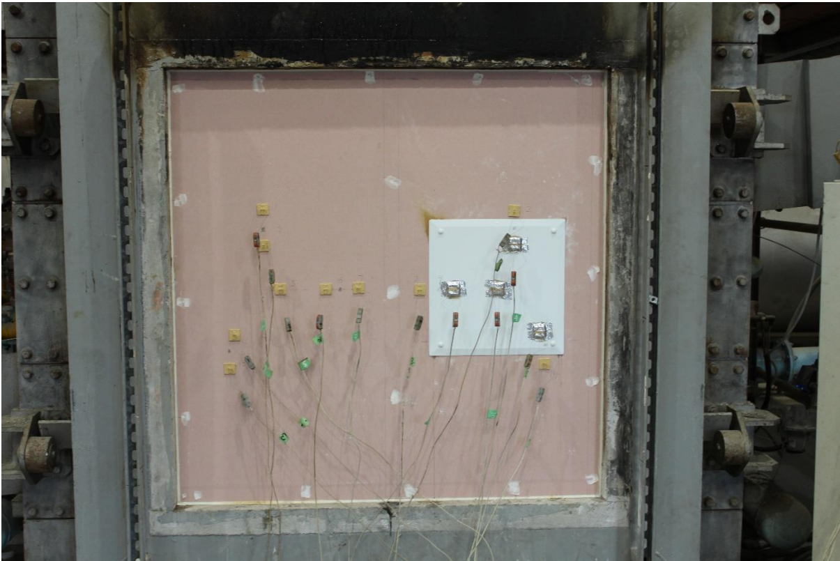
Figure 11 – Unexposed face at 30 minutes
